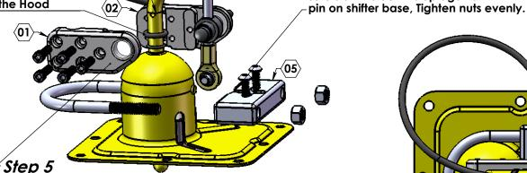
Assemble #01 & #02 onto Shifter, with 5 screws, using a 3/16" Hex Key.
